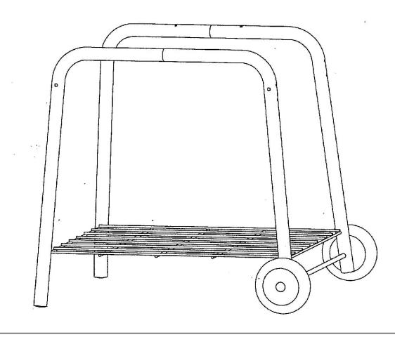
Install leg braces (item #7), with support flange towards center of grill, onto the legs using eight M6 x 15mm Phillips head bolts.
